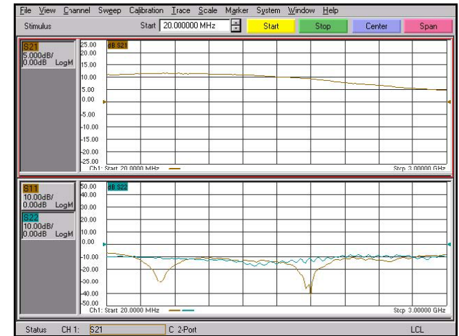
Swept Data & Noise Figure show typical performance across 20 MHz to 3 GHz frequency band.
